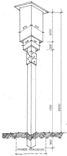
Typical Detail Double Chambered Rocket Box
